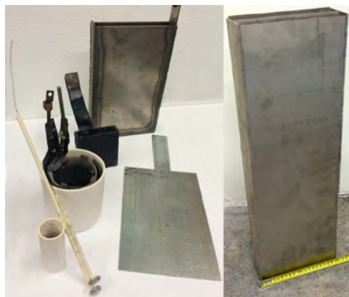
Figure 8. The evolution of the electrolysis chamber. Earlier versions can be seen in the front on the left, and later versions in the back and to the right. The rectangular electrolysis chambers use the interior walls as the air electrode (Licht, 2017).
