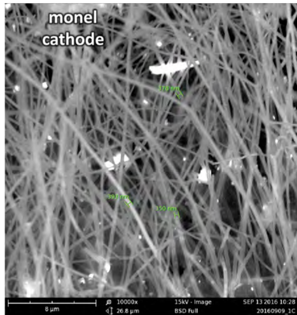
Figure 3. Comparison of the CNT product formed respectively at a copper (left side) and Monel (right side) cathode during short duration 0.3 \text{ Ah cm}^{-2} electrolysis in 770^\circ\text{C Li}_2\text{CO}_3 .
