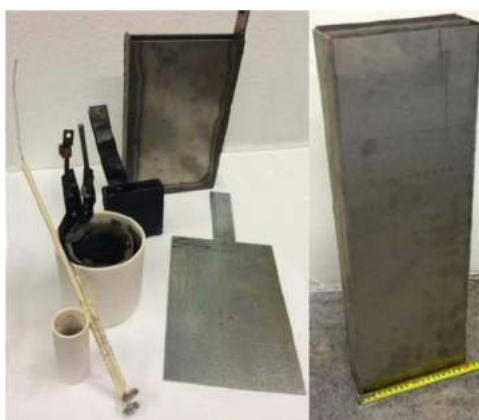
Fig. 8. The evolution of the electrolysis chamber. Earlier versions can be seen in the front on the left, and later versions in the back and to the right. The rectangular electrolysis chambers use the interior walls as the air electrode.
